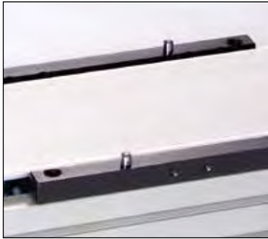
Two locating dowel pins shown in carriage
