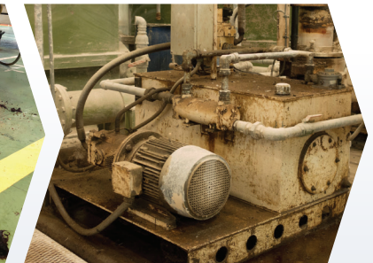
Constantly Running HPU Wastes Energy
